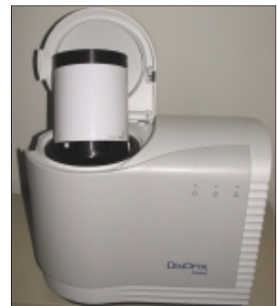
Fig. 2B: DenOptix™ (Dentsply/ Gendex, Des Plaines, IL) laser scanner with phosphor plate attached to drum ready for processing.
