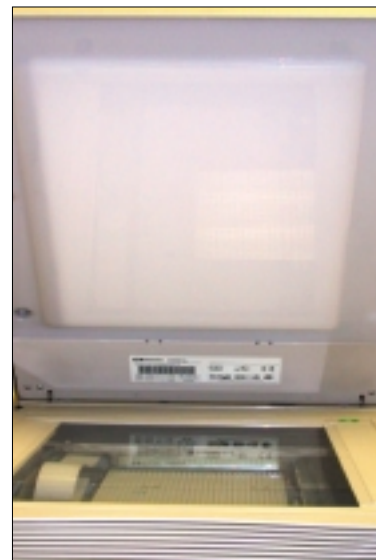
Fig. 1: Nikon CoolPix™ scanner with transparency adaptor in lid sufficient for extraoral radiograph duplication.
