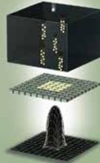
With Panoramic CdTe technology X-rays are not converted to light; therefore, no blurring occurs increasing clarity and contrast.
