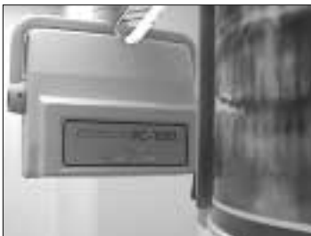
Fig. 6. The panoramic latent image is created as the film cassette moves past the secondary slit. The production of the latent image is simulated using the print of a panoramic radiograph.
