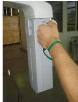
3. Remove the sensor carefully.
