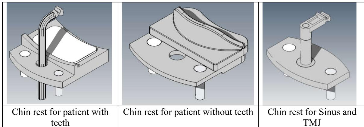
The first one is used for a patient with teeth and it has three parts (bite guide, chin rest and a silicon chinrest cover). The second is used for a patient without teeth and it has two parts (chin rest support and a plastic chin rest). The third is used for both kinds of patients (with or without teeth) for only the Sinus and TMJ profiles.
