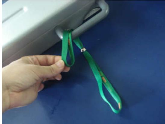
Pass the first strap loop inside the sensor handle.
